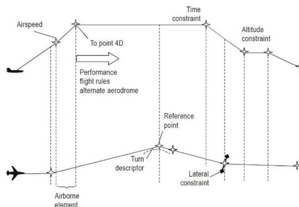
Figure 2: Airborne Segment of 4DT
