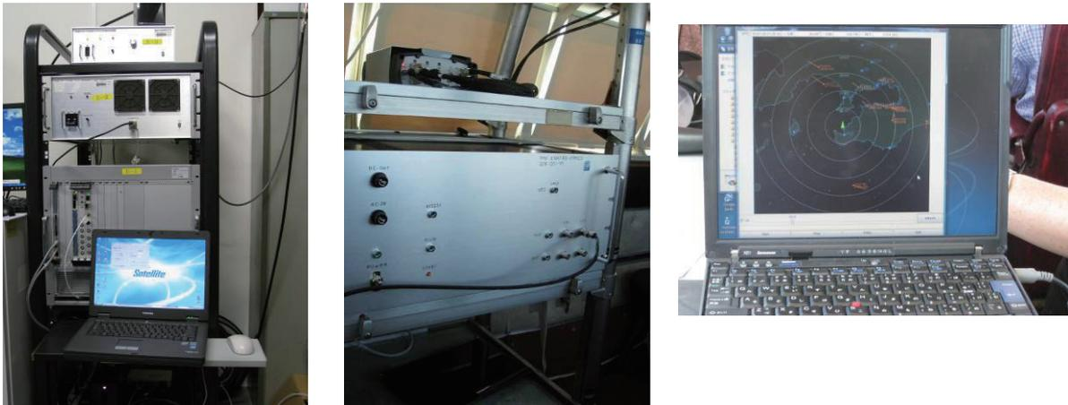
Fig. 7. ENRI prototype TIS-B system. The left is the ground station, the center is the ADS-B/TIS-B receiver on the aircraft, and the right is the PC-based data display.
