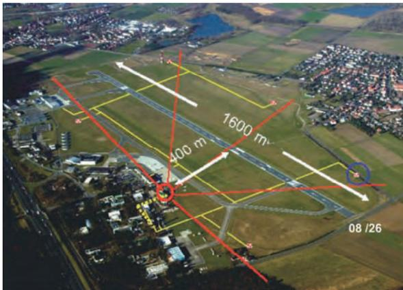
Fig. 2: Braunschweig research airport BWE with 1.67 km runway 08/26 extending E-W, fiber optic data link (thin yellow lines) connecting sensor containers. Circle with radiating lines indicate panorama camera position and sectors respectively.(Photo: DLR)
