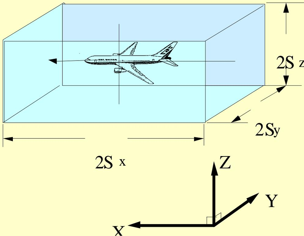
Separation minimum of aircraft pairs for tactical collision avoidance.
