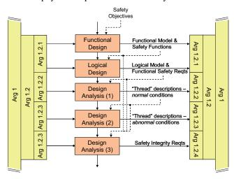
Fig 14.: Safety Assurance in Design & Validation Phase
