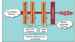
Fig 2: Simple ATM Barrier Model
