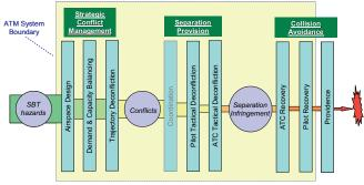
Fig 13: En-route / TMA Barrier Model
