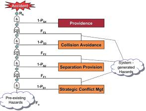
Fig 3: Fault Tree Version of Barrier Model
