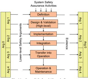
Fig 11: Overall Safety Lifecycle Process
