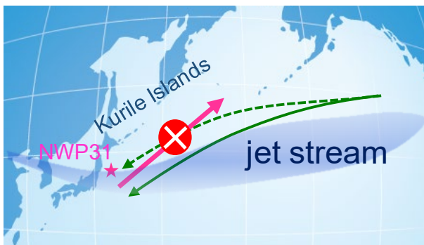
Figure 3. Route trends of westbound flights from North America to Japan and South Korea. Dashed green line indicates the ideal route that avoids jet stream core area (shaded) and is available in NOPAC FRA. With fixed NOPAC routes, flights cannot cross the NOPAC eastbound fixed airway (pink line) and hence must use the solid green line route.
