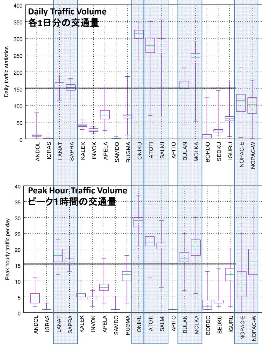
Analyse flows through main radar-controlled boundary points + NOPAC.
