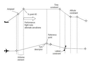
Figure 2: Airborne Segment of 4DT
