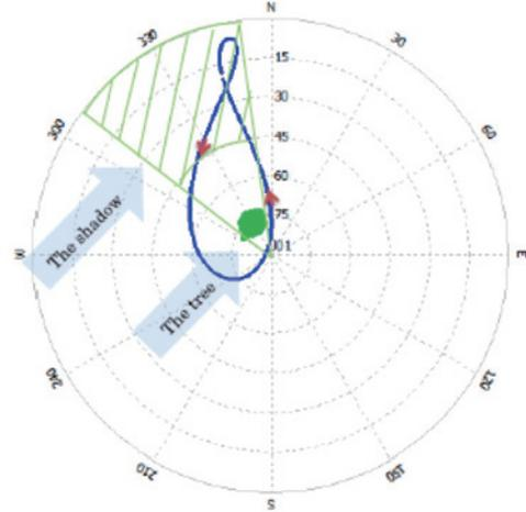
Figure 7 The signals attenuation under the tree shadow
