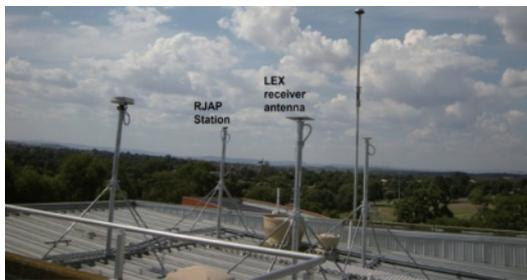
Figure 2 Antenna setup at Melbourne station
