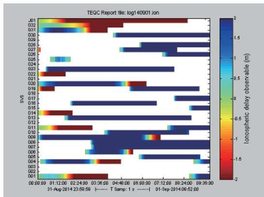
Figure 9 Ionospheric delay of L1-SAIF from QZS on Day 2014-09-01 at Melbourne station
