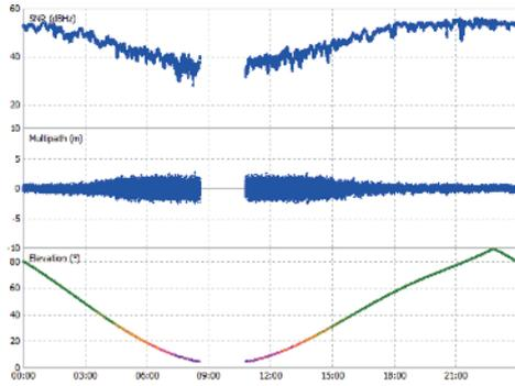
Figure 6 Visibility of L1C of QZS on 2014-09-01 at Melbourne station
