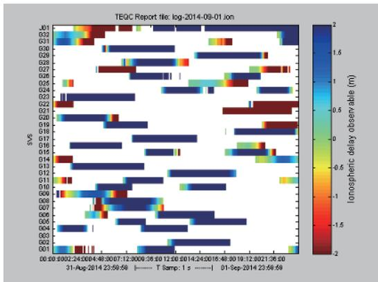
Figure 8 Ionospheric delay of L1-SAIF from QZS on Day 2014-09-01 at Sydney station
