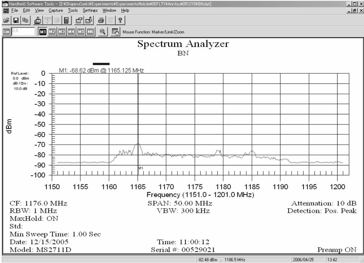
Figure 2 Measured power spectrum with two cascaded BPFs
