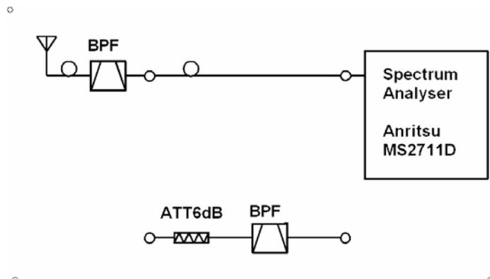
Figure 1 Equipments for onboard measurement
