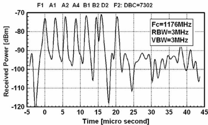
Figure 4 Interference by ATC transponder in L5/E5 band measured with 3MHz-BW
