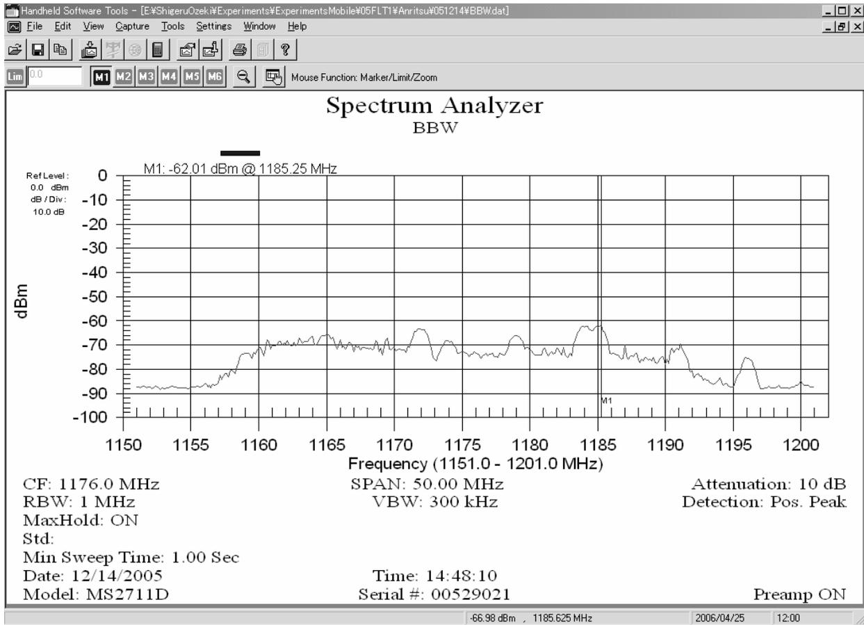
Figure 2 Measured power spectrum with a BPF
