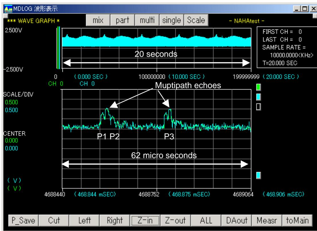
Figure 2, Zooming in to observe each interrogation signal pulse
