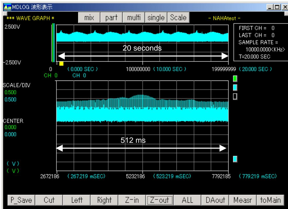
Figure 1 Example of received waveform in 1030 MHz channel at the Sendai Airport
