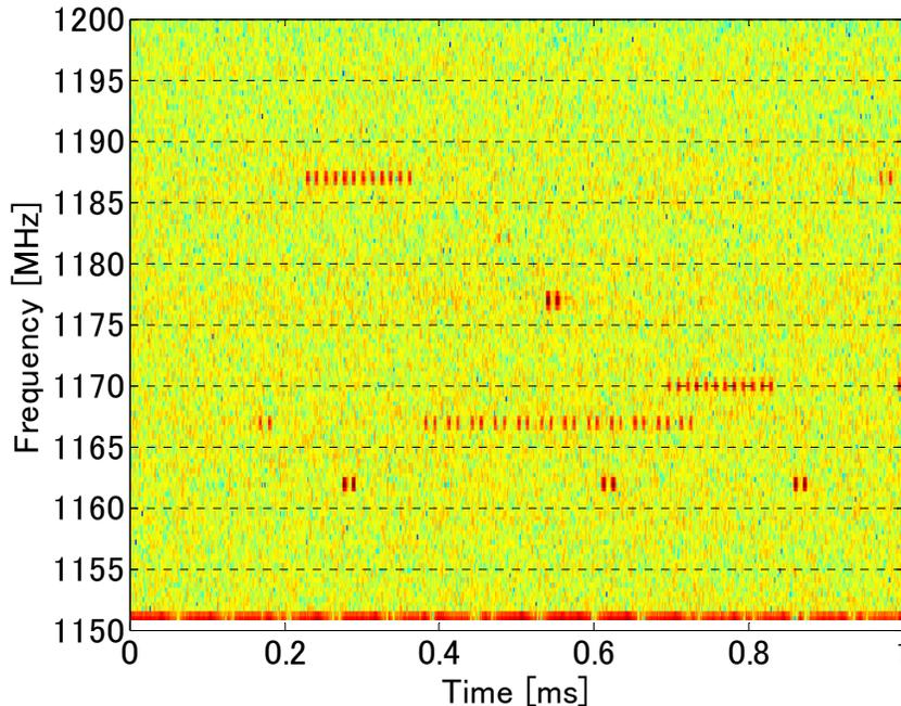
Figure 3, Measured power spectrum with a BPF
