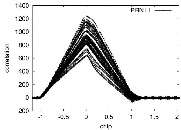
Figure 7: example of correlation curves of a signal with a reflective wave
