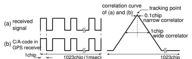
Figure 1: GPS signal and the correlation curve
