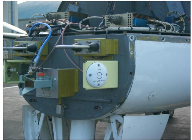
Figure 6: Photo of the GPS antenna attached into a nose of the experimental aircraft
