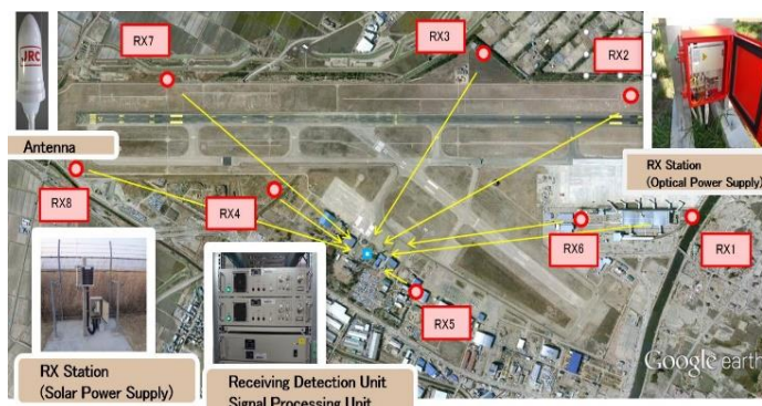
System configuration in the Phu Quoc
