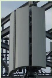
The ADS-B/MLAT sector antenna having high gain & small co-channel interferences could improve the signal reception performance for ADS-B and WAM (Wide Area Multilateration).
