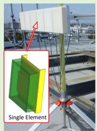
The patch array antenna developed for experimental purposes could contribute to achieve AOA accuracy of standard deviation 0.8° in the initial experiment for opportunistic ADS-B signals.
