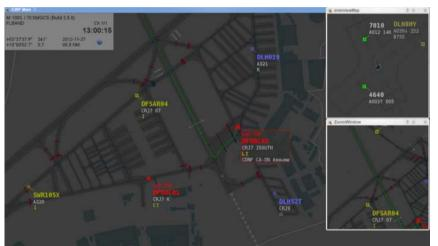
Detection of runway incursion and infringements of restricted areas by aircraft and vehicles and alert to the ATC controllers and vehicle driver.
