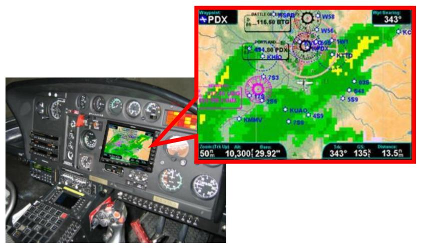
FIS-B transmits graphical National Weather Service products, temporary flight restrictions (TFRs), and special use airspace
