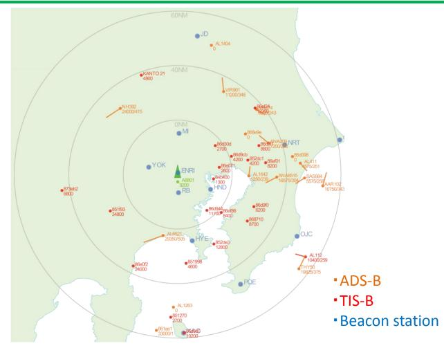
Simplified data plot from received ADS-B/TIS-B messages while airborne. The green triangle at the center indicates the airborne position measured by GPS. Red points indicate TIS-B aircraft, orange points with bar indicate ADS-B transmitting aircraft.
