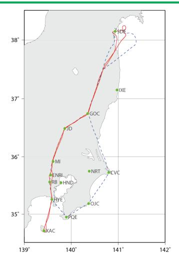
The flight route and beacon stations. Solid line indicates round trip route between Sendai(SDE) and Oshima(XAC). Dashed line indicate Kanto route.
