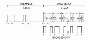
Fig. 4. 1090MHz extended squitter format
