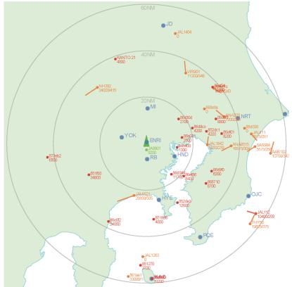
Fig. 9. Simplified data plot from received ADS-B/TIS-B messages while airborne. The green triangle at the center indicates the airborne position measured by GPS. Red points indicate TIS-B aircraft, Orange indicate ADS-B transmitting aircraft.
