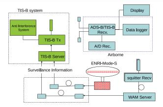
Fig. 6. The diagram of ENRI prototype TIS-B system.
