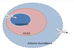
Fig. 1. Range of airborne surveillance
