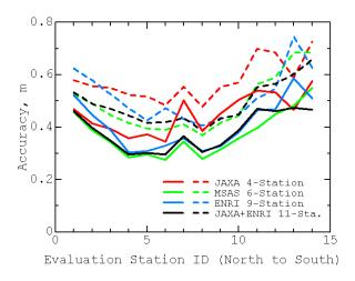
Figure 7 User position accuracies at evaluation sites for four configurations of monitor stations for 4 days; Solid and broken lines represent horizontal and vertical errors, respectively.
