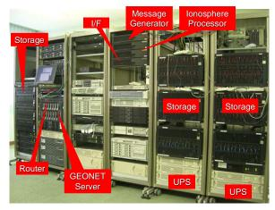
Figure3 L1-SAIF Master Station (L1SMS)
