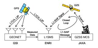
Figure 1. Experimental system configuration of QZSS L1-SAIF augmentation.
