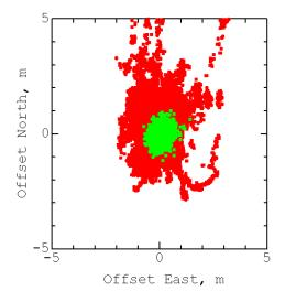
Figure 6 User position error at Site 940058 Takayama for Jan/19/08-Jan/23/08; (Green) Augmented by the L1-SAIF of 6-Station Config.; (Red) Standalone GPS.
