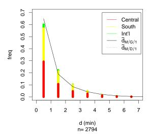
Figure 5 Observed and theoretical frequencies of metering delays.
