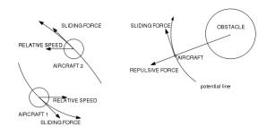
Figure 1 Principle of navigation functions between two aircrafts (left), between an aircraft and an obstacle (right)
