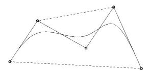
Figure 2 Control points, its convex envelope, control polygon and resulting B-spline
