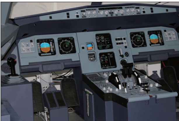
Figure 1 Displays and Instruments of the A320 Cockpit Simulator
