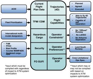
Figure 1 - Flight Object Data Example
