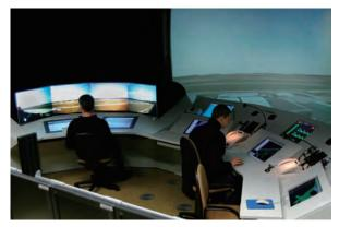
Fig. 11: RTC simulator environment. Photo of the  $200^{\circ}$  vision system of DLR tower simulator (ATS) with extension by the  $180^{\circ}$ -RTO console, showing live Panorama. Photo: DLR.
