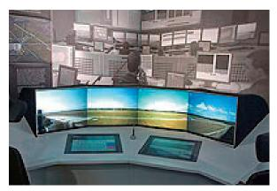
Fig. 3: RTO HMI for  $180^{\circ}$  single airport surveillance, integrating videopanorama. Backprojection displays for cameras no. 1=W-4=E, PTZ display below (right), and pen touch-input interaction display (left) integrated in the table.(Photo: DLR)
