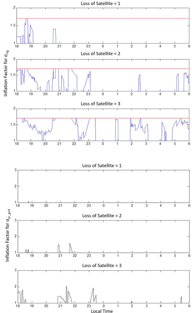
Figure 5. Inflation factor for  $\sigma_{vig}$  (top) and  $\sigma_{pr\_gnd}$  (bottom)
