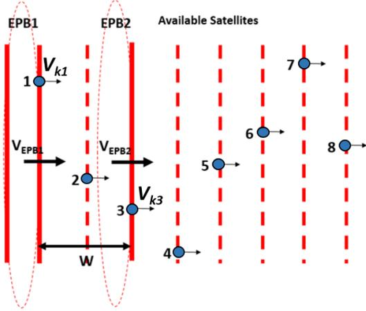
Figure 3. Double-satellite impact scenario by different EPB
