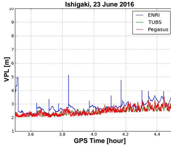
Figure 4. VPL values generated by derived by ENRI-Airborne, TriPos, and Pegasus software for the data from 03:30 to 04:30 GPST on 23 June 2016.
