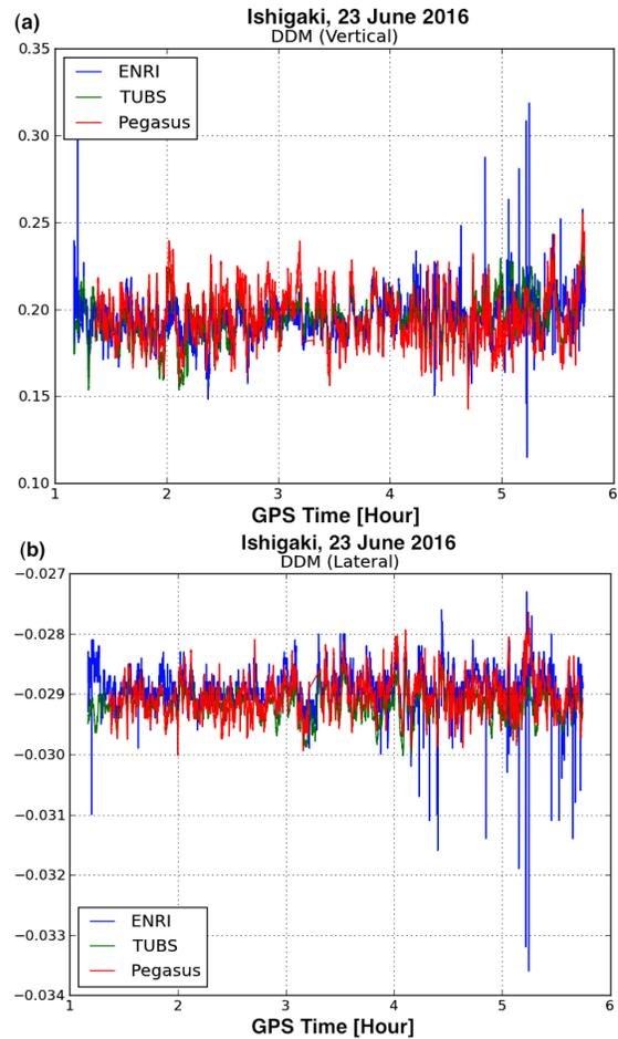
Figure 2. (a) Vertical and (b) lateral DDM values, respectively derived by ENRI-Airborne, TriPos, and Pegasus software for the data on 23 June 2016.
