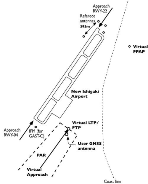
Figure 1. Geometry of measurements at New Ishigaki Airport.
