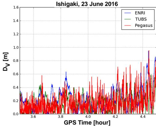
Figure 3.  $D_V$  values generated by derived by ENRI-Airborne, TriPos, and Pegasus software for the data from 03:30 to 04:30 GPST on 23 June 2016.
