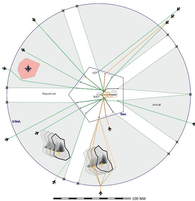
Figure 4 Schematic representation of the presented airspace structure with Extended Terminal Maneuvering Area (E-TMA), Aircraft Separation Points (ASP), and Late Merging Points (LMP) for each runway (RWY). Green lines represent individual negotiated and optimized approach routes, orange lines standard routes.
