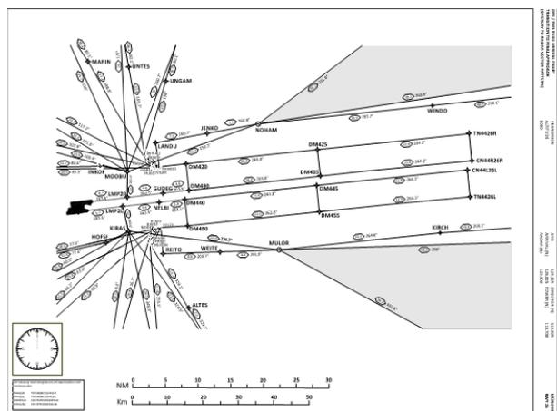
Figure 6 Airspace structure with LMPs, trombone path stretching area and finals as airspace map.
