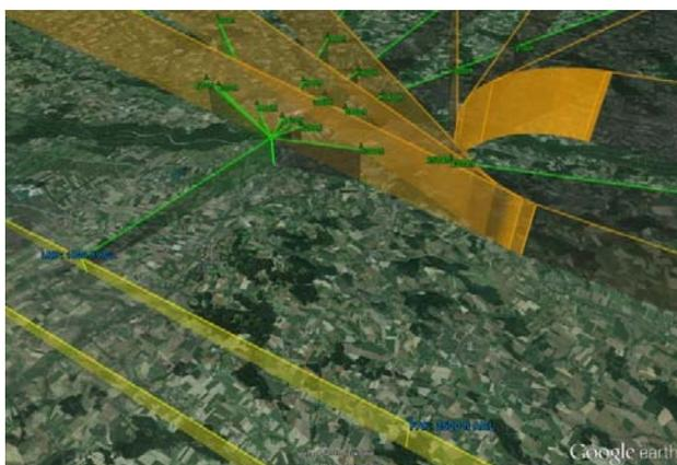
Figure 5 3D model of the standard arrival routes for CDA (green) and conventionally equipped (orange) aircraft with average separation values (green triangles), final approach depicted in yellow [12].
