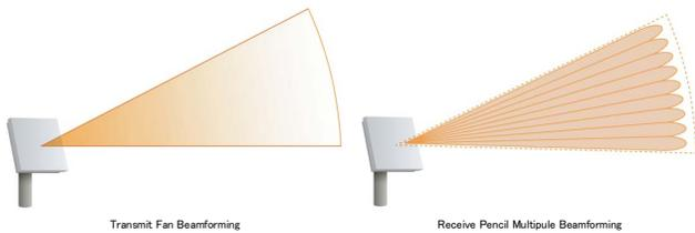
Figure 3. Transmit and receive beamforming.
