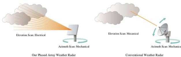
Figure 2. Differences of volume scan between phased array weather radar and parabolic weather radar.
