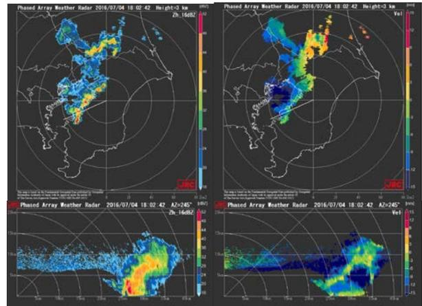
Figure 8. CAPPI at 3 km and RHI at 246 deg of the convective system, July 4, 2016. Figures of left side indicate the reflectivity and figures of right side indicate the doppler velocity.
