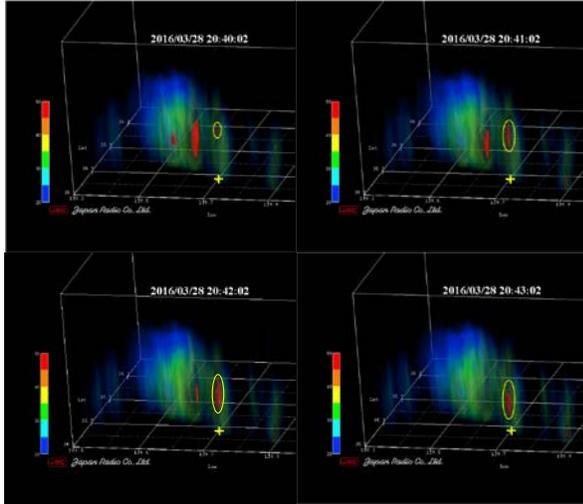
Figure 6. Time-series 3D images of reflectivity of a thunderstorm on March 28, 2016. The marker indicates Shinjuku.
