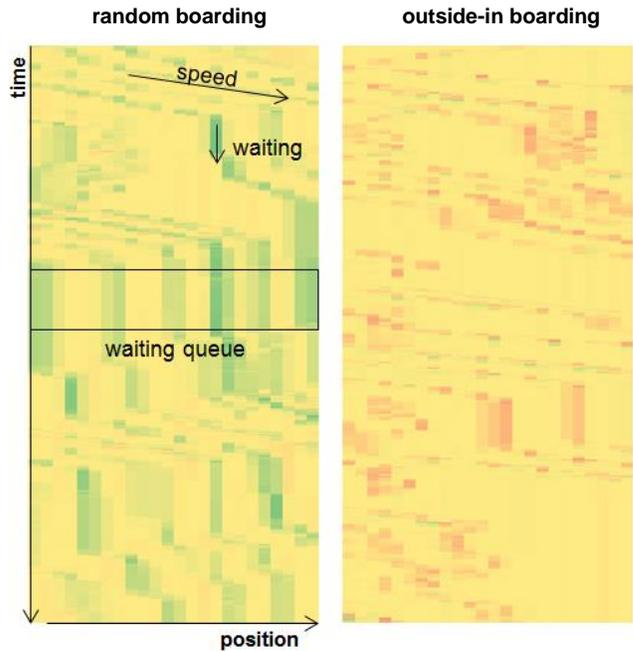
Figure 16. Feedback from the floor sensors indicating walking speeds and passenger queues in the aircraft cabin.
