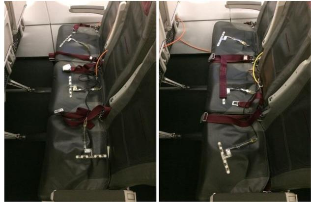
Figure 15. Seat sensors in a field trial environment (Schultz, 2017c).
