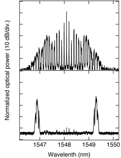
Figure 2 Obtained optical spectra of (top) FM-CW-signal-launched optical frequency comb and (bottom) two-tone signals passed after the OFB.
