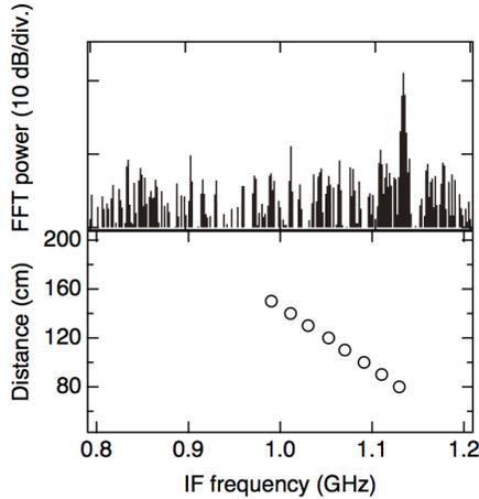
Figure 4 (top) IF spectrum obtained by FFT of digitized Rx signal and (bottom) ranging results with various target distances.
