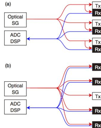
Figure 1 Concept of terahertz-band multistatic radar system under (a) TRx and (b) TX-Rx separation configurations. Red and blue arrows denote an LO and RF signal lines and IF lines, respectively.
