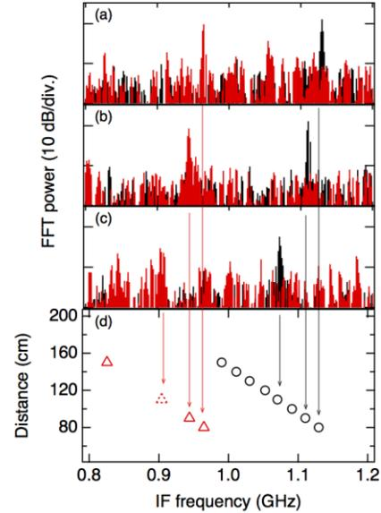
Figure 5 (a-c) (a-c) IF spectra obtained by FFT of digitized Rx signal with several target distances and (d) ranging results with various target distances. Red and black lines and circles show obtained signals from different Rx.
