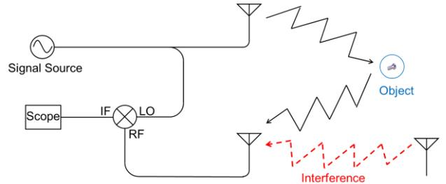
Figure 4 Basic FMCW radar diagram
