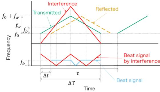
Figure 2 Linear cell radar diagram
