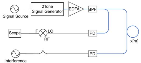
Figure 5 Experimental setup diagram of FMCW radar
