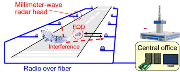
Figure 1 Linear cell radar diagram [2-5]
