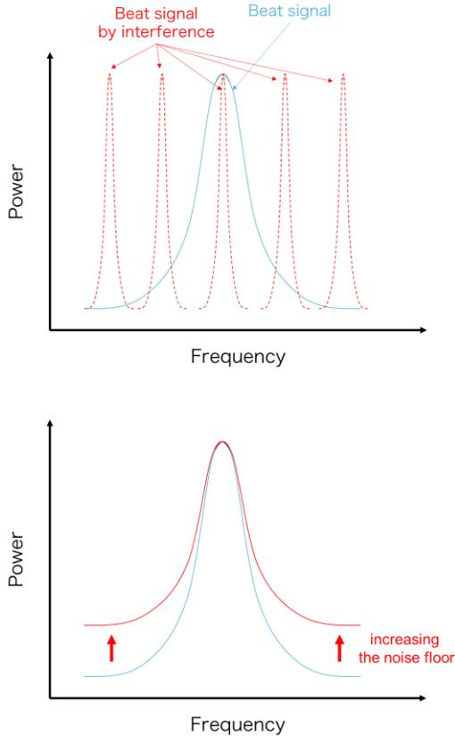
Figure 3 Mechanisms of FMCW radar interference
