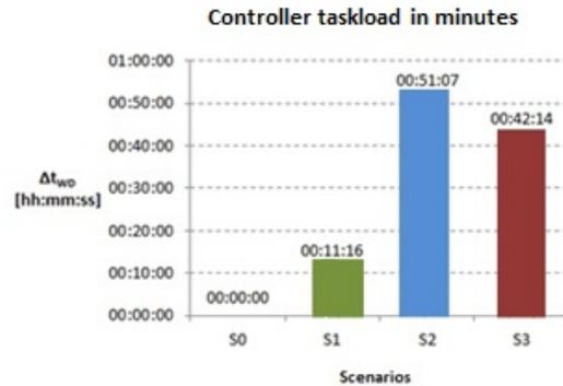
Chart 3 Controller taskload calculated (min) [2]
