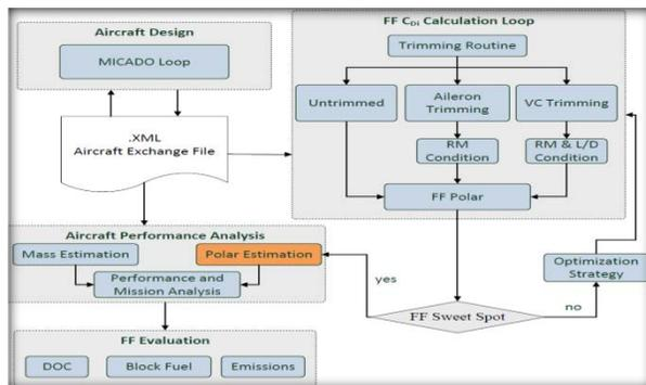
Figure 3: The overall process of aircraft formation flight modelling at the ILR, RWTH Aachen
