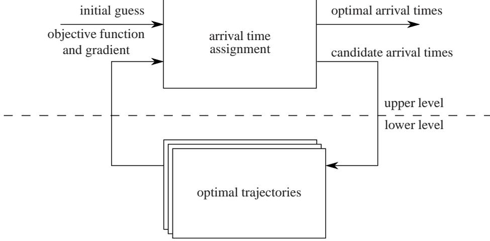
Figure 1: Bi-level structure resulting from the primal decomposition of the multi aircraft approach problem.
