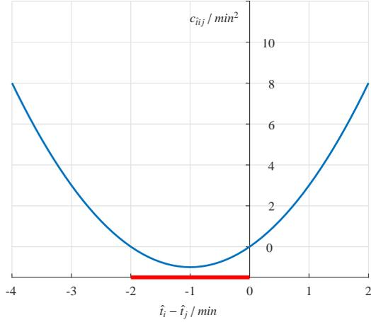
Figure 2: Combined time separation constraint function between aircraft  $i$  (H) and  $j$  (M).
