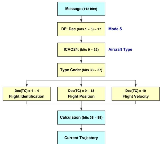
Figure 4 Message decoding for current trajectory updating
