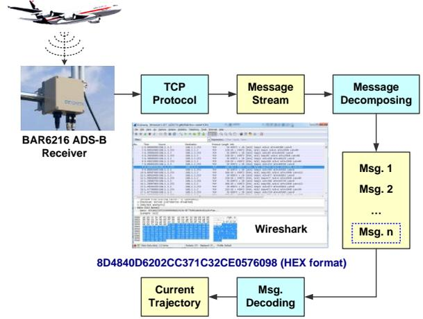
Figure 3 Processing steps for current trajectory updating
