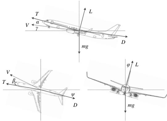
Figure 2 Diagram of forces acting on an aircraft
