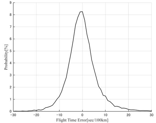
Figure 2 Histogram of Flight Time Error at 100km (N=33791)
