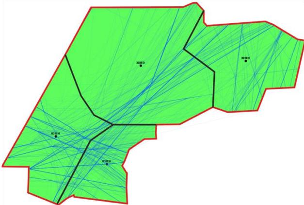
Figure 8 Airspace EDDYDUTA with air traffic movements (aircraft trajectories) as blue lines with the current existing sectors. A darker blue color represents a higher traffic density on the trajectories.
