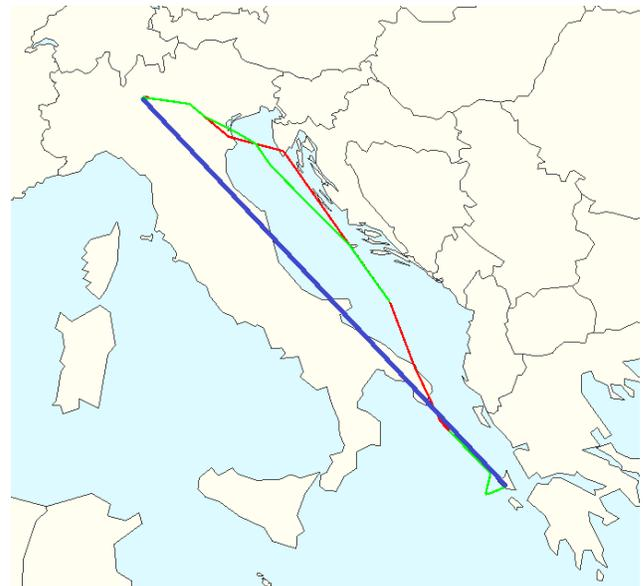
Figure 2 Difference in planned (red), actual (green) and direct (blue) trajectory of a flight from Bergamo to Corfu.
