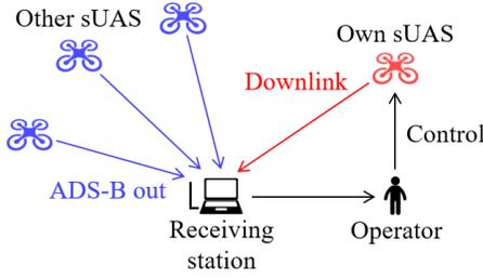
Fig. 1 Implementing configuration of ADS-B.
