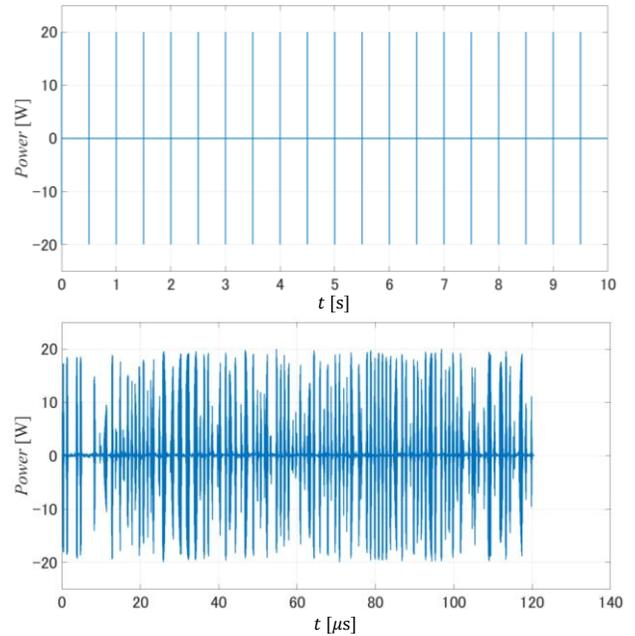
Fig. 5 Actual ADS-B signal used in the simulation. (bottom: magnified one extended squitter signal)
