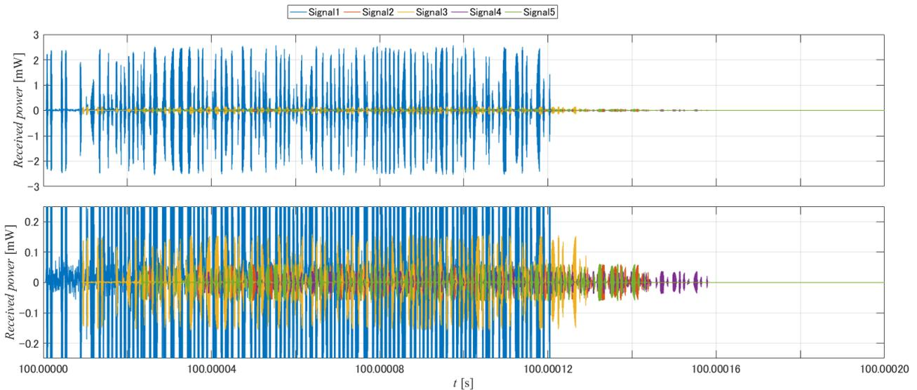
Fig. 7 Estimated ADS-B signals at the receiving station. (bottom: magnified figure)
