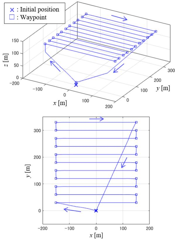
Fig. 3 Flight path of the single sUAS. (top: in 3D; bottom: in 2D)
