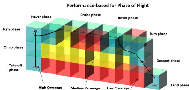
Figure 3 Sample schematics of safe flight path based on phases of flight
