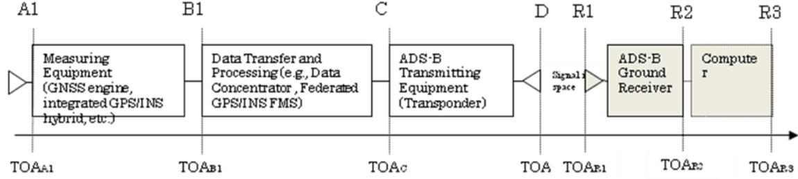
Figure 1. Functional architecture diagram with general timing
