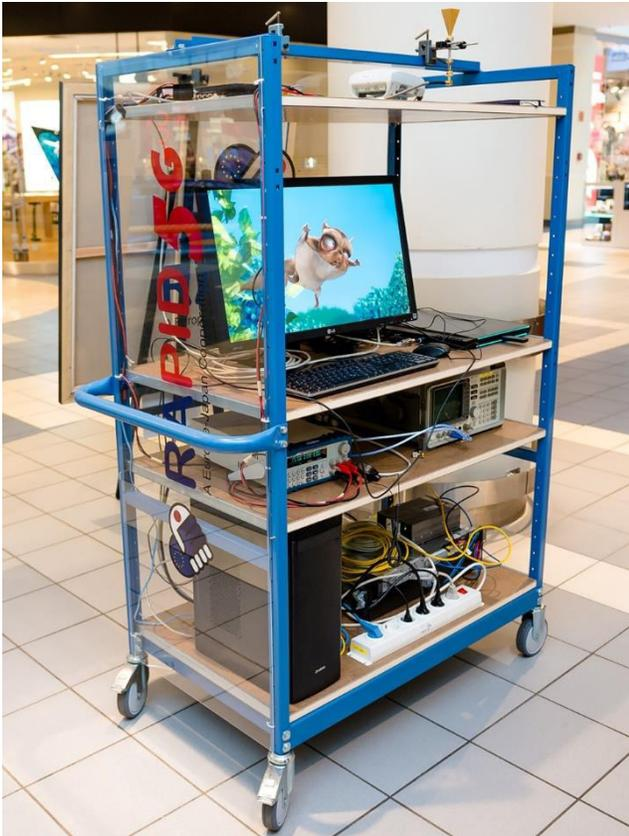
**Figure 7** RAPID5G demo vehicle as mobile user in the shopping mall, containing a receiver horn antenna, a RF amplifier, a SBD detector, a baseband amplifier a SDI-to-HDMI scalerbox and a 4K high resolution screen to display the received video stream.
