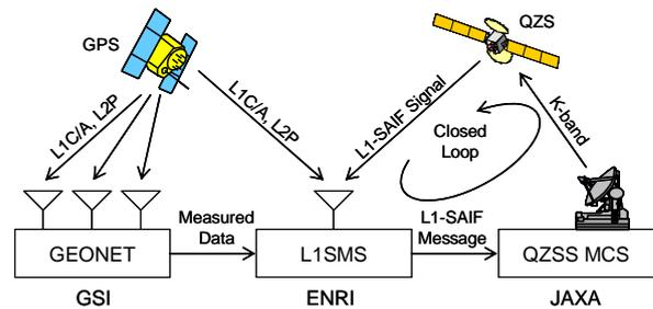
Figure 1. Experimental system configuration of QZSS L1-SAIF augmentation.
