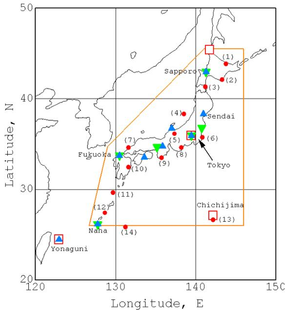
Figure 5 L1-SAIF experimental area (bordered by orange line; (Red Square) JAXA monitor stations; (Green Triangle) MSAS GMS; (Blue Triangle) ENRI real-time sites; (Red Circle) Real-time test user stations numbered with brackets.
