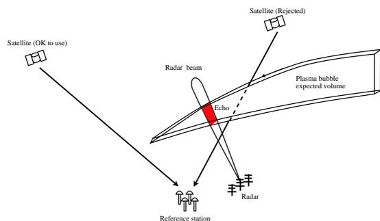
Figure 6 Principle of radar monitoring of plasma bubble.
