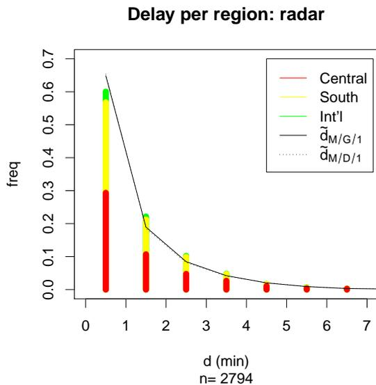
Figure 5 Observed and theoretical frequencies of metering delays.
