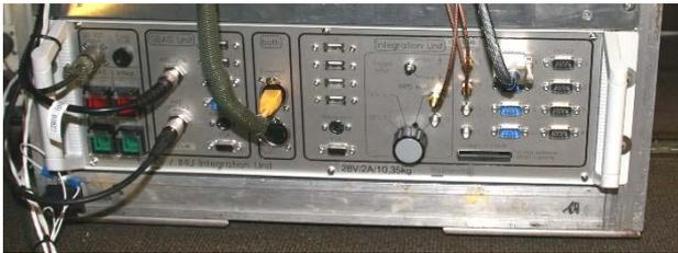
Fig. 4: GBAS/INS integration unit (Funkwerk Avionics)
