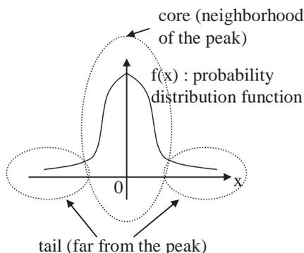
Figure 5 Core and Tail of Distribution
