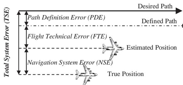
Figure 4 Lateral Navigation Error<sup>[7]</sup>
