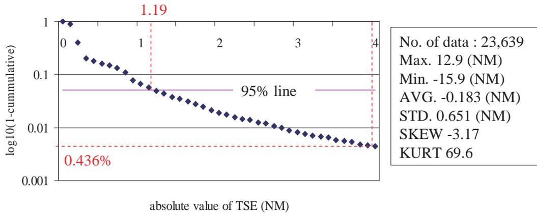
Figure 7 TSE observed at the middle point between NUBDA and NANNO (Oct. 2006 – Sep. 2007)
