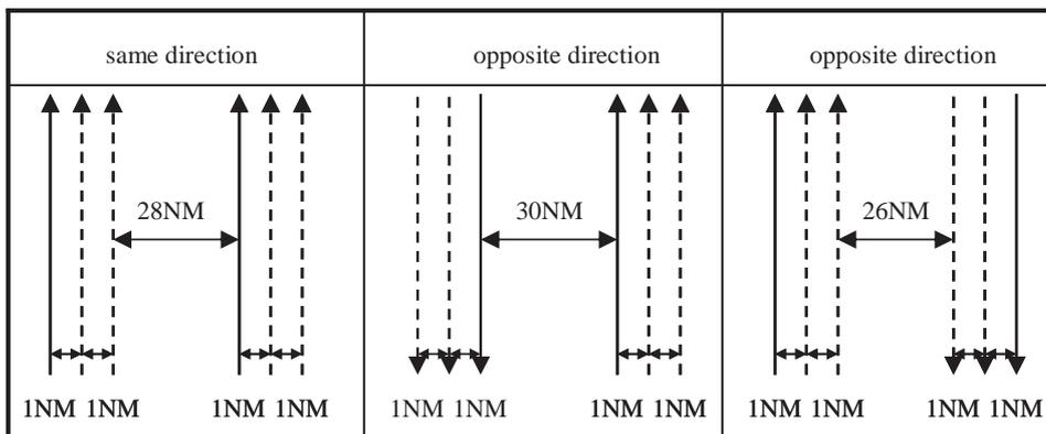
Figure 3 Effect of SLOP to Route Spacing (30NM nominal route spacing)
