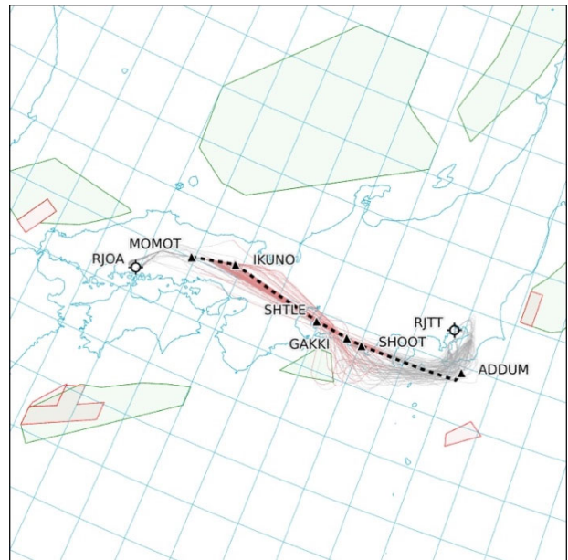
Figure 6 Flight tracks (grey lines: below FL310, red lines: above FL310) and most common flight plan route (dashed black line) of flights from Hiroshima airport (RJOA) and Tokyo Haneda airport (RJTT) during a week in 2019.
