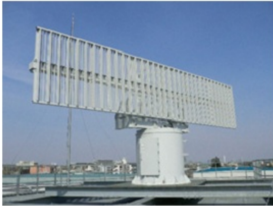
Fig. 1 ENRI's experimental Mode S SSR.
