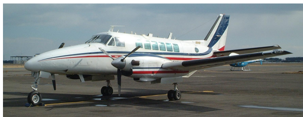
Figure 1: ENRI's experimental Aircraft Beechcraft B99 Airliner A VHF antenna for receiving GBAS-VDB is mounted on fore part of a roof. A GPS receiving antenna is mounted on rear of the VHF antenna.
