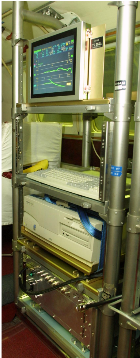
Figure 8: Experimental GBAS airborne subsystem top: LCD display middle: PC for GBAS processing bottom: GBAS-VDB receiver
