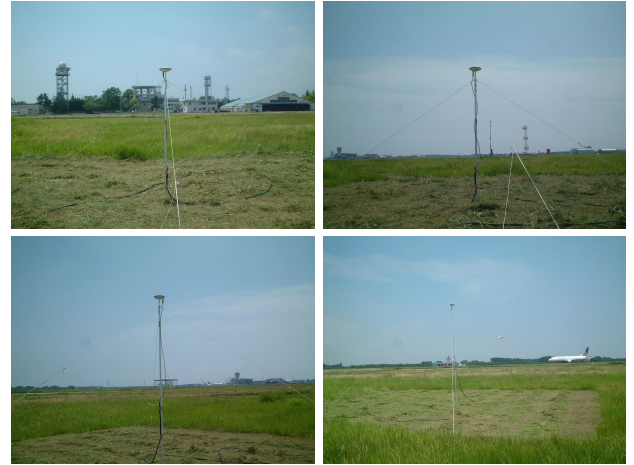
Figure 4: Reference GPS antennas Each height of antenna was 1.7m (upper left), 2.0m (upper right), 3.0m (lower left), 4.0m (lower right).
